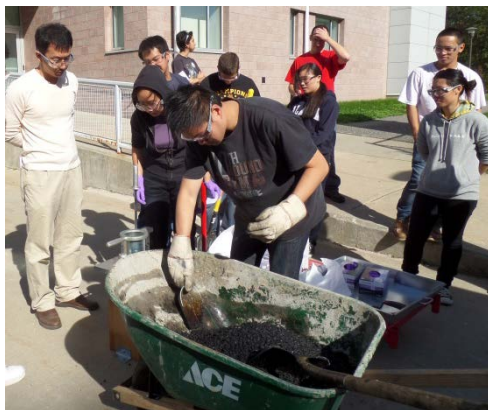
Yuanchun Lu scooping out hot asphalt to prepare Marshall Stability Test samples.
