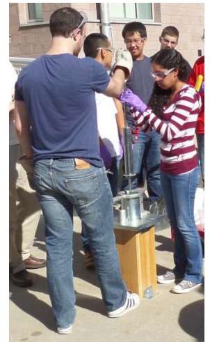
Gabby & her classmates making an asphalt sample for the Marshall Stability Test in CIV Materials Lab, fall 2014
